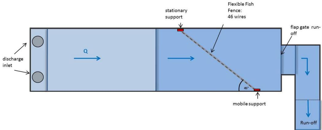
**Figure 3** Layout of the model test
