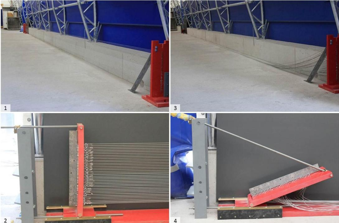
**Figure 2** Flexible fish fence in operation mode (1 and 2); released mode of flexible fish fence (3 and 4)
