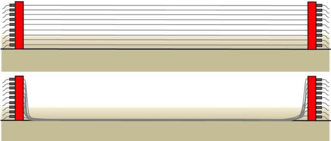
**Figure 1** Operating mode and released mode of the flexible fish fence
