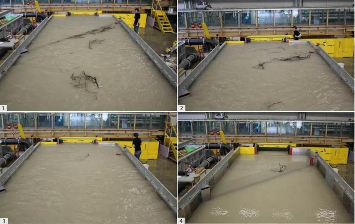
**Figure 8** Test with branch input: (1) initial state, (2) relaxation of the wires, (3) transition to operation mode, (4) final state after cleaning
