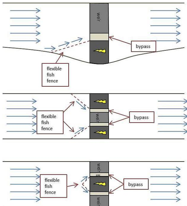
**Figure 9** Layout of the flexible fish fence at different hydro power plant arrangements
