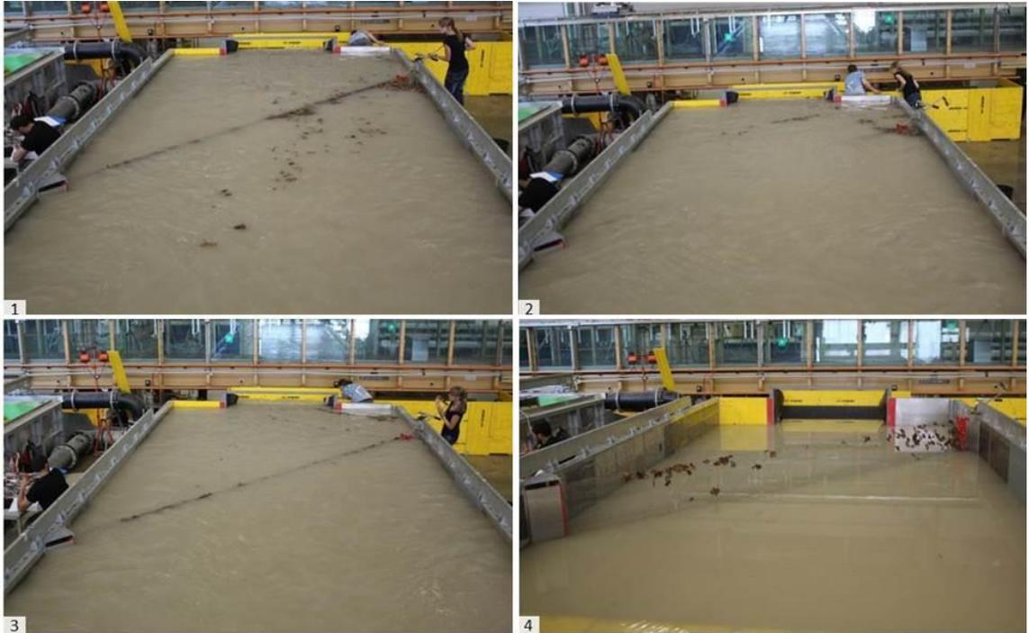
**Figure 7** Test with leaf input: (1) initial state, (2) relaxation of the wires, (3) transition to operation mode, (4) final state after cleaning
