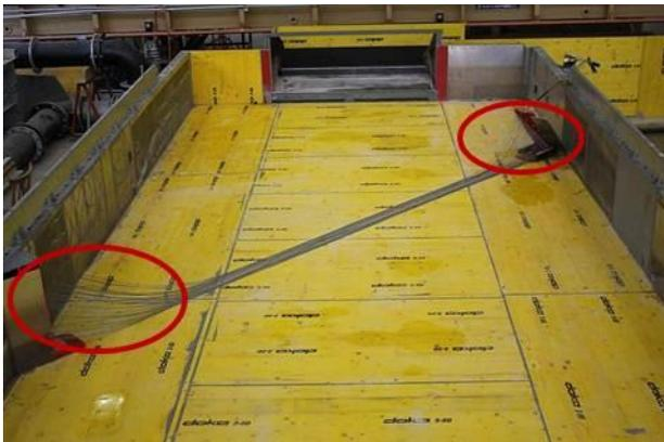
**Figure 5** Released mode of the model test fish fence
