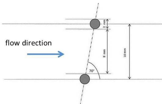
**Figure 6** Optimization of the wire arrangement
