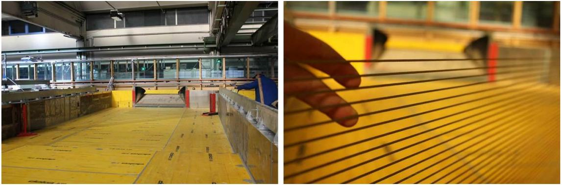
**Figure 4** Model test fish fence in operation mode
