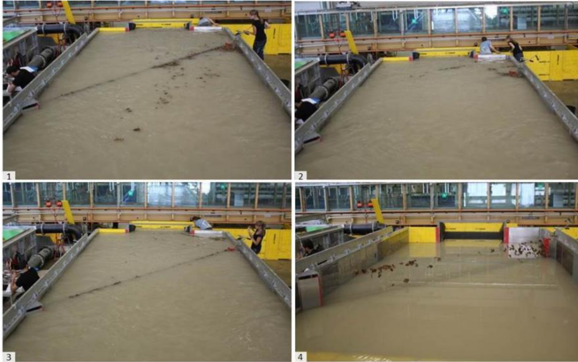
Figure 3 Test with leaf input: (1) initial state, (2) relaxation of the cables, (3) transition to operation mode, (4) final state after cleaning
